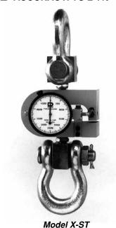
CAPACITIES: 100 TO 10,000 LBF Model X-ST comes in seven capacities for tension testing; all are equipped with a maximum load pointer. Force is applied through spherical rod end fittings on models to 2000 pounds and with shackles and pins on 5000 and 10,000 pound models. The X-ST is available in pound or kilogram capacities.
