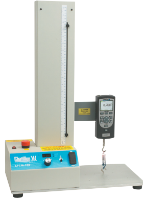
DFs II gauge mounted to LTCM100 tester
