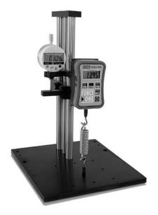
Force One™ FDIX shown mounted on Wagner FTK 100 Test Stand
