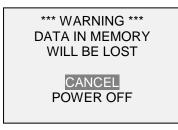
If no option is selected, this screen will be displayed indefinitely, or until battery power has been depleted.
