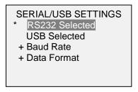
Select either RS-232 or USB input (output is always active for both the USB and RS-232 ports). Communication settings are permanently set to the following:
