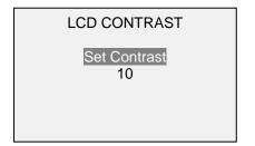
Press ENTER to modify the contrast. Select a value from 0 to 25, 25 producing the most contrast.
