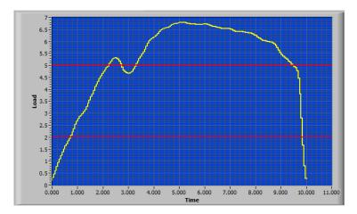
MESURgauge and MESURgauge Plus plot load versus time or load versus travel, depending on the system configuration. X-axis and Y-axis minimum and maximum values can be changed by double-clicking on the numerals along the axes. When the numeral is highlighted, type the desired value, then press **ENTER** or click away from the area.
