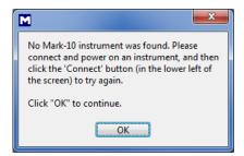
If the instrument is properly connected and configured but this message still appears, the COM port connection may be manually configured. Refer to the communication flowchart below and the following sections for details.
