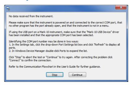
This message appears after clicking **START** if communication has not been achieved between the instrument and the software, due to a number of possible causes. Refer to the communication flowchart in the **Startup** section. If following these instructions does not resolve the issue, consult with an IT administrator.
