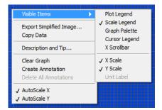
The menu items are provided for quick access and convenience to some common functions. The *AutoScale X* and *AutoScale Y* items are equivalent to the "padlock" icons in the *Scale Legend*, as described below.
