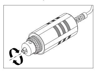
Fig. 3.1 Proper axial loading of Series TT03 torque gauge.
